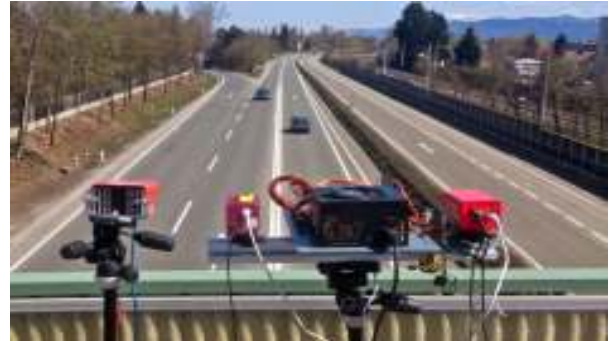
Figure 1: Our vision based traffic monitoring system under power management [32]
