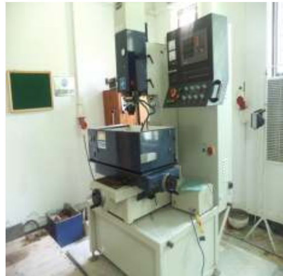
Fig.2 Electrical Discharge Machine (EDM) Die Sinker
