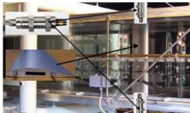
Figure 1: View of the wind tunnel test section. The black arrows indicate the installed position of strain gauge force sensors and the vertical airfoil [16].
