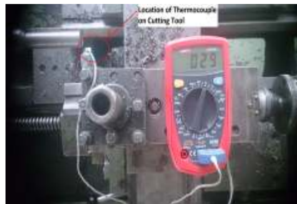
Fig.3 Thermocouple arrangements on tool
